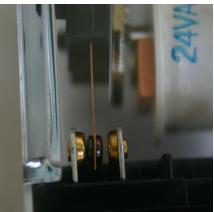
The high-magnification photo at the far right shows the contacts on this relay. The lefthand contact is NC; the righthand contact is NO. The magnet is wrapped in white tape, marked 24VAC in blue lettering. Eight screws in the black base are used for electrical contacts (2 to power the magnet, 2 for the higher voltage power supply, and 4 for the NO and NC contacts). If the relay burns out, simply unplug it from the base and install a new relay.
