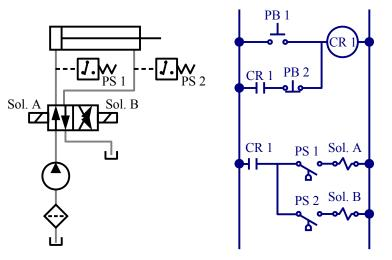
This circuit could be automated in other ways. For example, you could use limit switches in place of pressure switches, or you could use timers.
