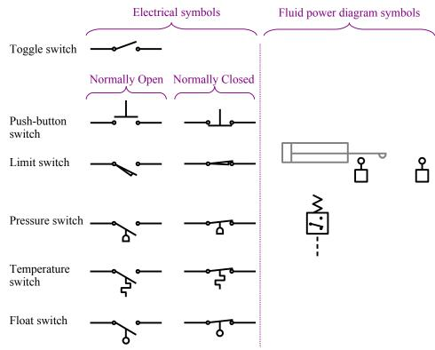
contacts and the switch below the contacts. Consider the left-hand contact point a hinge; the switch rotates counterclockwise up when actuated. The NC symbols develop a gap when the switch lifts.
